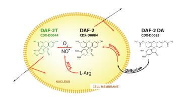
**FIGURE:** The cell-permeable diacetate derivative DAF-2 DA is used to load cells. Subsequent hydrolysis by cytosolic esterases releases DAF-2, which is relatively non-fluorescent at physiological pH. However, in the presence of NO $^{\circ}$  and O $_{2}$ , DAF-2 is converted to the fluorescent triazole derivative DAF-2T.
